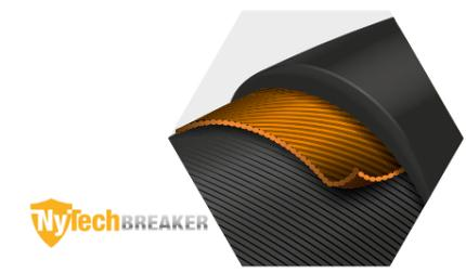
**Light and sleek** The Nytech Breaker is based on the technology of our SafetySystem puncture protection. Made of nylon fibre and similar to Kevlar, it reliably protects against punctures and cuts. It also has particularly low rolling resistance and reduced weight, perfect for our performance range of road tyres.
