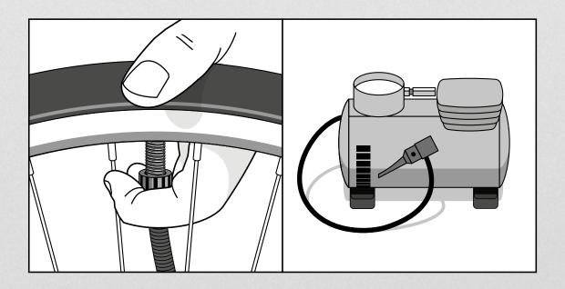
To fit the tire between the hooks, you 5 may need a higher amount of air in the first instance. If you are using a floor pump, it is better to maintain a constant momentum within the first few seconds. A modern floor pump with a second inflatable cartridge can help to achieve this.
