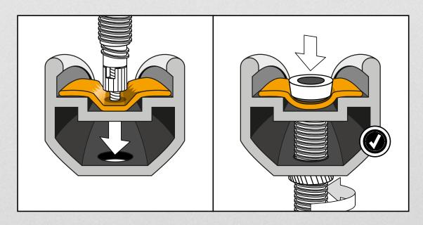
Mount the Tubeless valve first. 2 Install it from the inside of the rim and tighten the nut. Press your finger on the rubber end of the valve to secure a better fit. Only tighten the nut by hand, do not use any tools.
