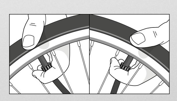
If you are using tire sealant: For in-9 flation place the tire with the valve at the 11 or 1 o'clock position. Otherwise sealant could leak into the valve or put too much turbulence into it. It could dry faster or lock up the valve core.
