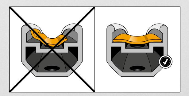
Check both rim and rim tape. Only use Tubeless ready rims. Ensure that the rim tape covers the rim well with at least two layers.
