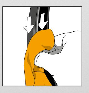
Before the initial inflation you can 3 apply some soapy-water or a mounting pad on the contact points between tire and rim bed. This can help improve mounting the tire on the rim.
