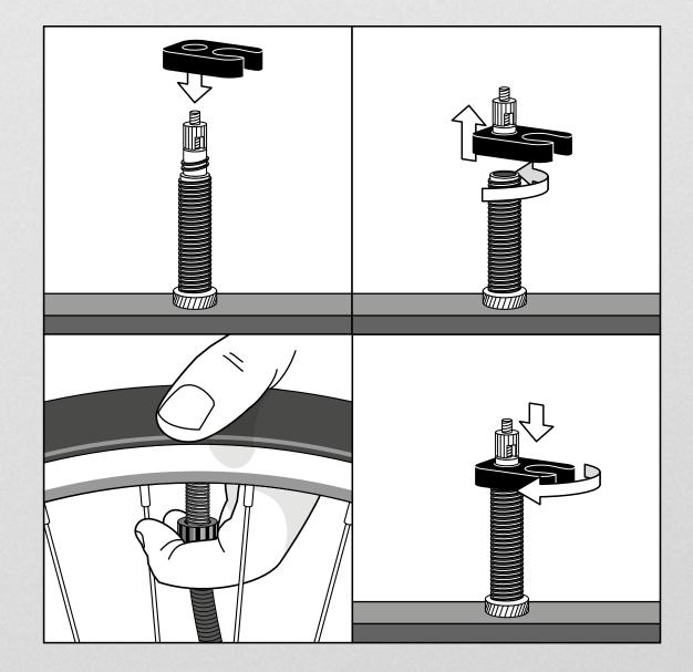
To enhance the air volume, unscrew 7 the valve core. Pump it up and screw the valve core in again.
