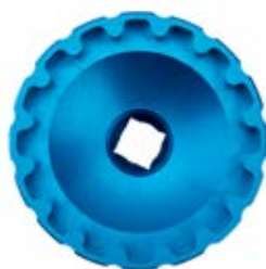
BBT-47-16 Fits 16-notch components Inner Diameter: 48.8 mm Outer Diameter: 52-54 mm
